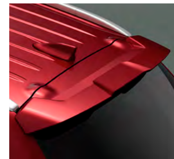
REAR SPOILER The rear spoiler has been optimised to further improve aerodynamic performance.
