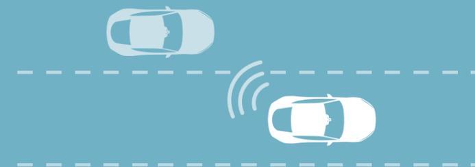
**Blind Spot Assist Pack** (Optional<sup>10</sup>) can help you prevent collisions. If another car is in your blind spot when you begin to change lanes, Blind Spot Assist detects the car and applies corrective torque to encourage you to guide your vehicle away from the approaching vehicle. **Rear Traffic Monitor** uses the same system to alert you, via the Touchscreen, of moving vehicles during reversing.
